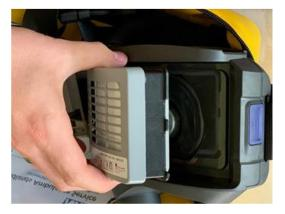
Step 1 - Check the status of the battery by pressing the 'Test' button. The battery will last for approximately 9-12 hours on standard flow and 9-10 hours on high flow. Battery chargers are provided with each unit. **NOTE: it is the responsibility of the person who has been individually issued the Powered Hood System to ensure the battery is charged.**
