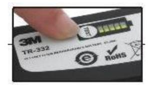
Step 2 - Check that the battery is securely fitted to the unit. If replacing the battery, the non-blue end must be placed in first and then closed next to where the blue clip is. You will hear an audible click to confirm. Do not force the battery into place, as this may damage the blue clip.
